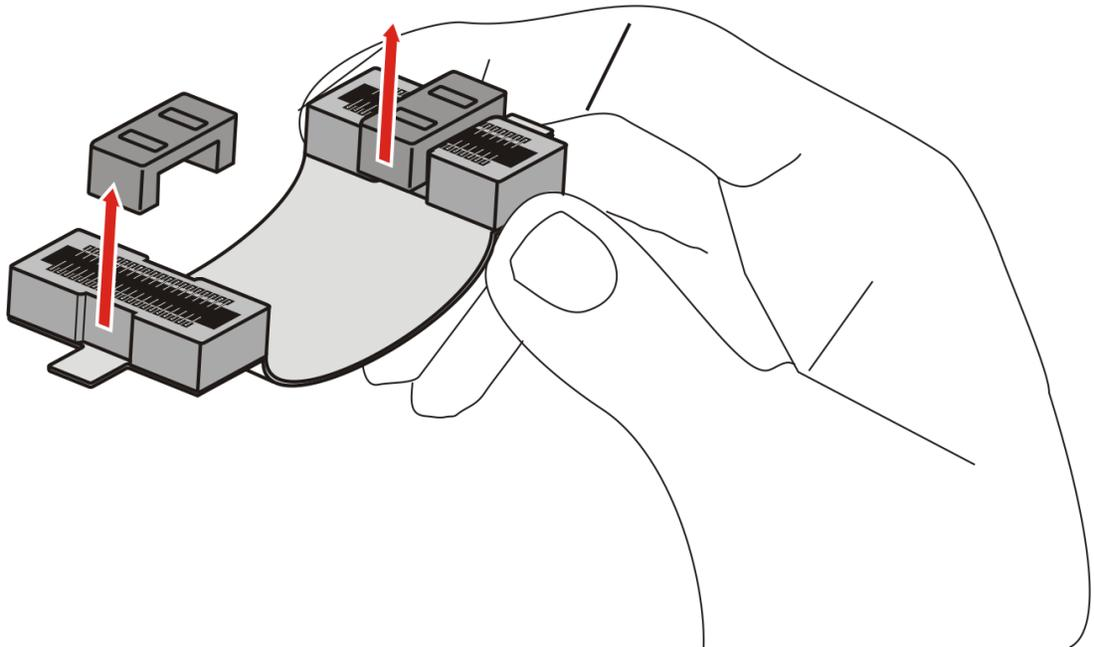
Figure 2–2 ATI CrossFireX Installation
